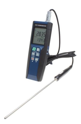
DTM-385 and DTM-386 are handheld RTD thermometers with extremely high measurement accuracy, suitable for low temperature measurement, and suitable for temperature detection that requires high measurement accuracy.
