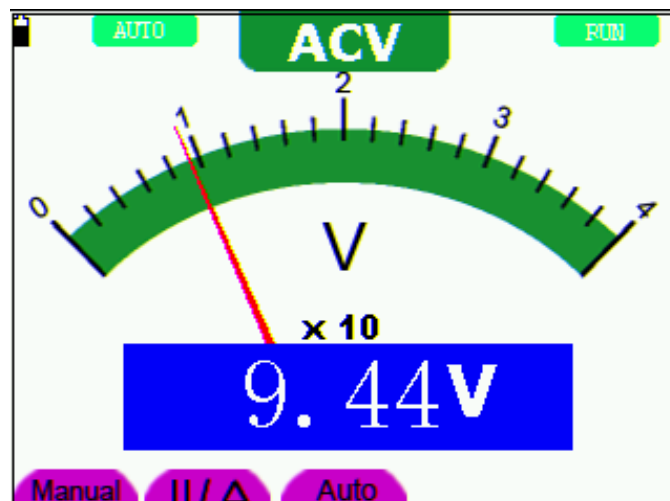
Figure 26: AC Voltage Measurement
