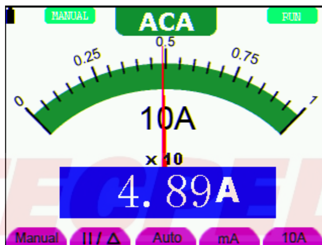
figure 30: AC Current Measurement for 10A
