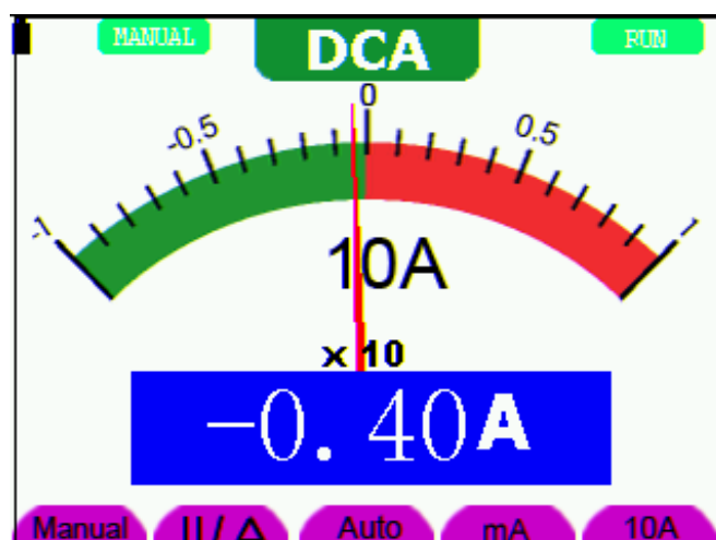
figure 28: DC Current Measurement for 10A
