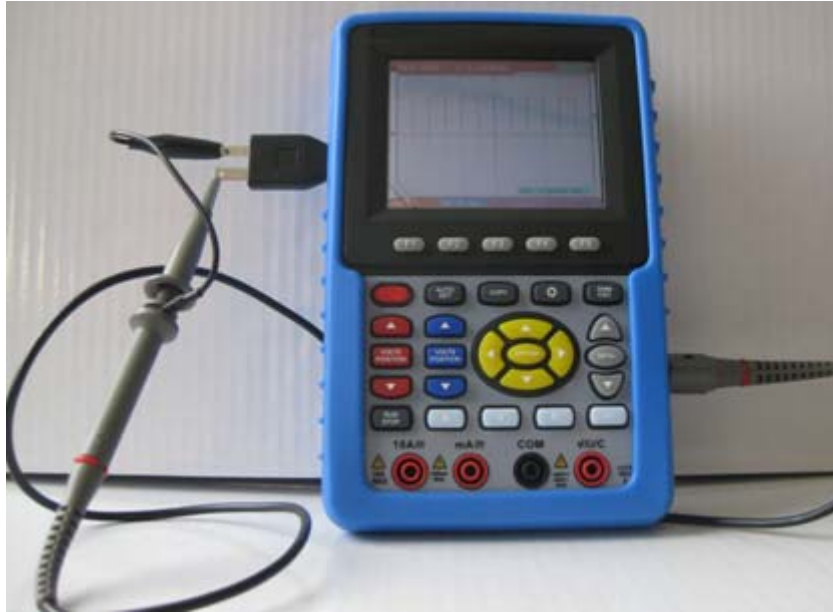
Fig.3. The connection of Square-wave test signal
