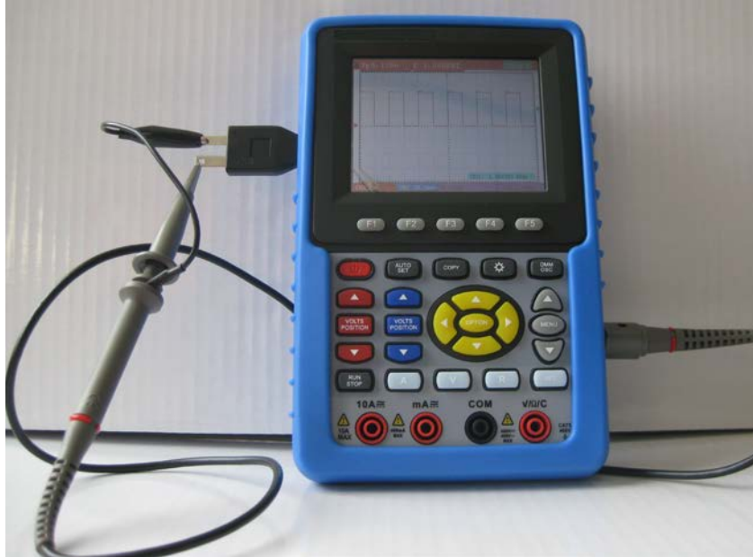
Fig.3. The connection of Square-wave test signal
