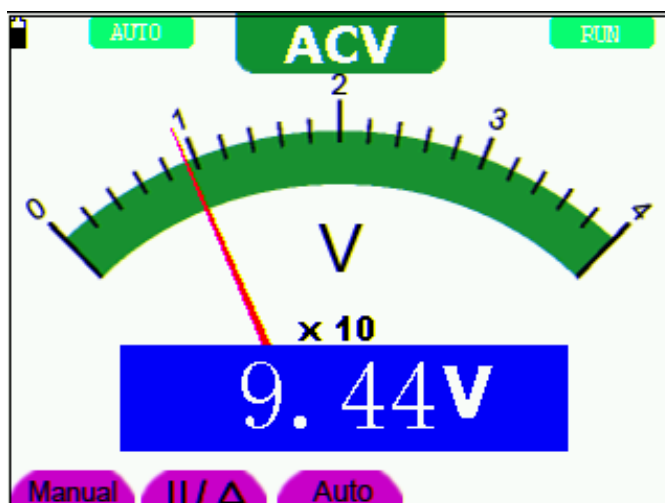
Figure 26: AC Voltage Measurement
