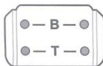
Note: There are two pairs of metal contacts on the top of the probe cap, which can be used to test the instrument. One pair of metal contacts is marked "T", and the other pair is marked "B".
