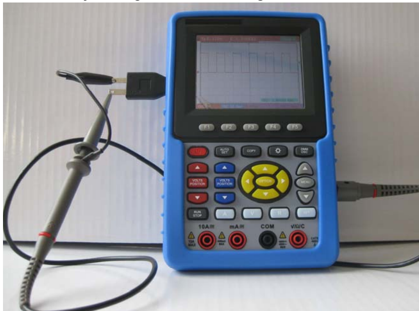
Fig.3. The connection of Square-wave test signal
