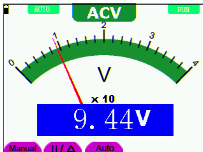
Figure 26: AC Voltage Measurement
