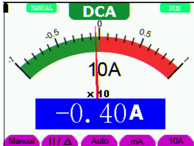
Figure 28: DC Current Measurement for 10A
