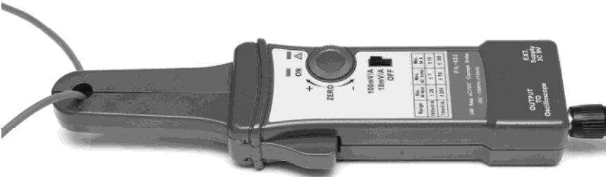
Figure 2: Connecting the PA-622 current probe.
